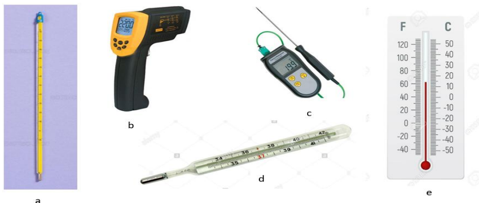
Fig-10.2, a) Mercury thermometer; (b) Radiation thermometer; (c) Thermocouple thermometer; (d) Clinical mercury thermometer; (e) Alcohol thermometer
