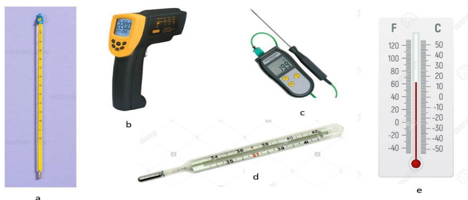
Fig-10.2.1, a) Mercury thermometer; (b) Radiation thermometer; (c) Thermocouple thermometer; (d) Clinical mercury thermometer; (e) Alcohol thermometer
