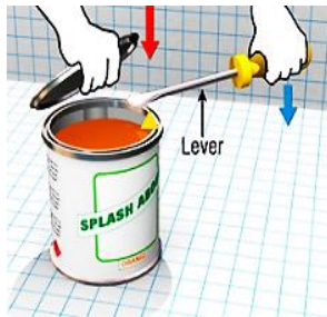
Fig- 6.7. Example of Class 1 lever.
