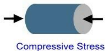
Fig-8.2(b), Compression Stress
