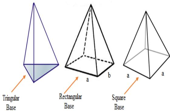
$$V = \frac{1}{3} \text{Area of the base} \times \text{Height} = \frac{1}{3} Ah$$
