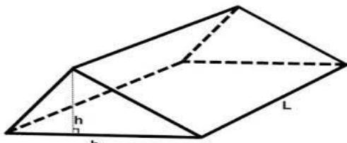
$$V = \text{Area of cross section} \times \text{Length}$$
